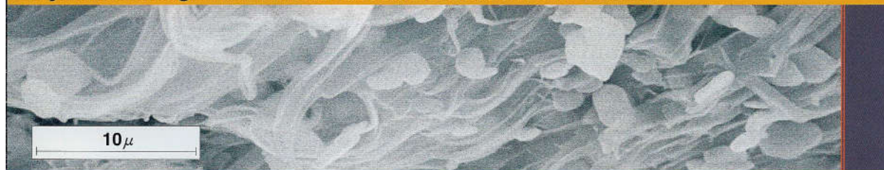
SEM photograph of a fractured PP surface filled with KISUMA 5
