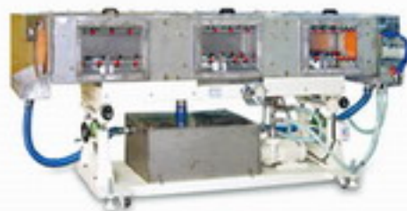
8" Spray Cooling Tank
